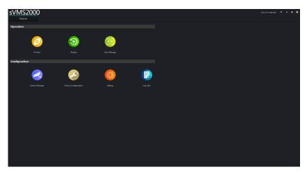
After entering correct login password, enter the homepage interface of the software. As shown in the figure, this software has seven functions: preview, playback, face management, device management, device configuration, setting and log. First, the user needs to click Device Management to add devices. Only after the devices are added successfully, can the user preview and configure in the software.
