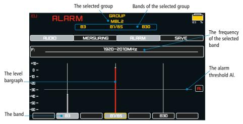
**The alarm threshold** can be adjusted, and the **ALARM** and **AUDIO** functions can be switched on. A subsequent **pressing of the joystick button** selects the BAND mode where a band can be inspected
