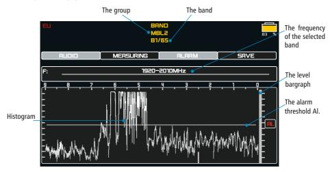
In addition to the level bargraph, a **histogram** is displayed in this mode. The histogram is a graph where the history of the signal level for a certain time period is shown. It allows you to not miss the signal when you approach, or move away from the transmitter, or when it has a non-continuous mode of operation.
