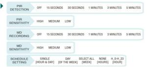
▶ PIR Detection/M.D. Recording: The duration of time, in seconds, that the DVR will countdown while continuing to record after motion has been detected, which triggers the recording process.
