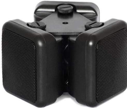
White noise generators are widely used for protecting premises against acoustic leakage eavesdropping. The SP2300 omnidirectional speaker is an important component for such system. While the transducers inject the generated noise into the surfaces and structures stopping distributing of sound through them, the role of the speaker is to fill voids, cavities and ventilation shafts with the audio interference to prevent leakage of sound through the air.
