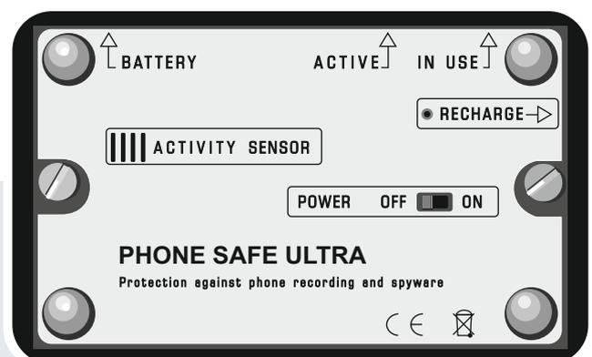
The orange, 'IN USE' LED on the right side, will indicate that a phone is installed in the device.
