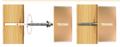
To avoid damaging the wire behind the transducer put the provided spacer ontothe screw or bolt before threading it in the surface, dowel or anchor.
