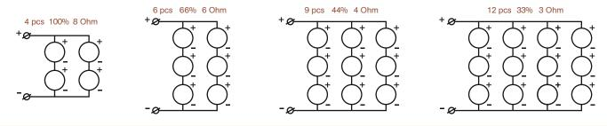
The output power is divided between the transducers, so when there are more transducers, each separate unit will receive less power. The percentage shows the relative power produced by a transducer, comparing to the variant with 4 transducers connected 2 x 2.
