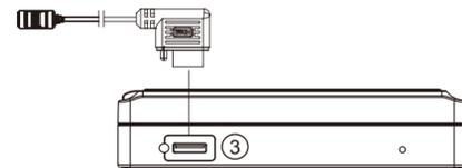
1. Plug in the Controller cable into the Control port (3).
