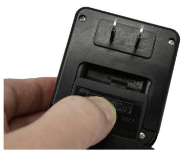
2. Install the memory card by inserting it until secured in the memory card slot. You should hear or feel a click once the slot secures the card. If it will not fully insert into the slot, flip the card over and try again. *Note: Forcing the memory card to be inserted in the improper orientation may damage the device and void the warranty.*
