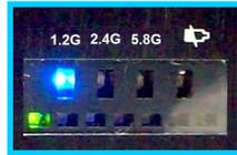
3.2 The lower row is indication of **scanning** and **image lock**. During scanning, the green LEDs will shuttle to-and-fro. When receive video signal, user can lock the image, then green LED will still.
