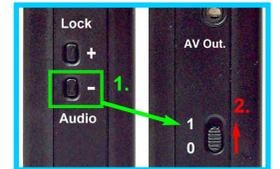
Press the (-) button in left side once, the warning mode will shift from 1. Beep and vibration → 2. Vibration → 3. Beep cyclic. After set the preferred warning mode, press both (+) (-) buttons to save your setting.
