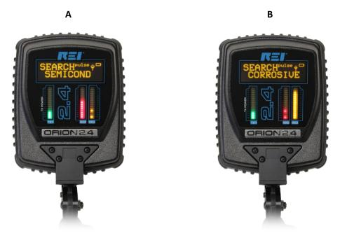
ORION 2.4 COMPARISON OF HARMONIC LEVELS (A – Semiconductor, B – False Junction; Bargraphs on the right are the 2<sup>nd</sup> and 3<sup>rd</sup> harmonic levels)
