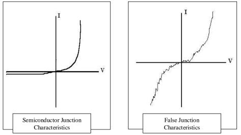
This level of regularity in the junction results in differences in the harmonic signals. When the ORION 2.4 radiates a signal that is returned by the junction in electronics, it results in a strong  $2^{nd}$  harmonic signal and a weak  $3^{rd}$  harmonic. A false junction returns a very weak  $2^{nd}$  harmonic and a strong  $3^{rd}$ .
