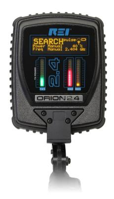
This document is intended to provide guidance and instruction on using the ORION 2.4 Non-Linear Junction Detector for finding hidden electronic devices.
