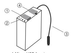
1.Micro USB Input 2.LED indicator light 3.DC Output 4.Switch
